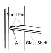
7. Insert Shelf Pins to desired height. Slide the Glass Shelf into position and tighten the plastic set screw (A)
